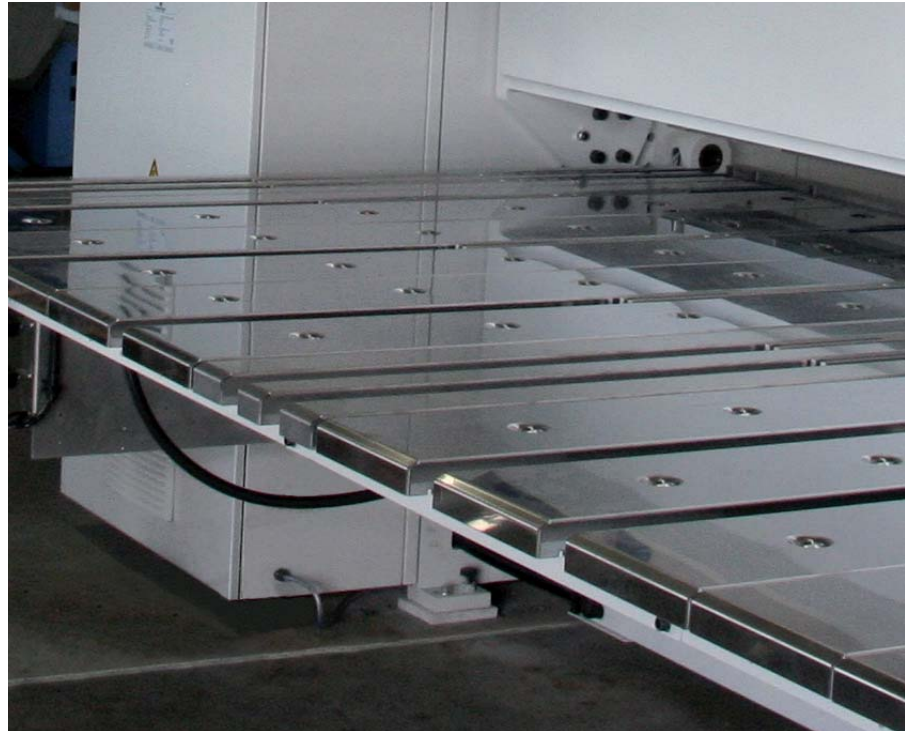
Gauge table, 1,600 mm, closed, with ball transfers
