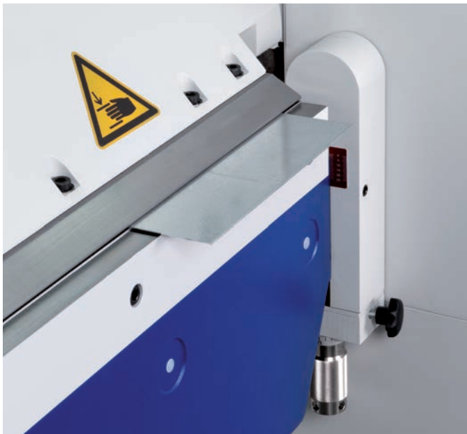
In the standard version, the MAKV is available with a tinsmith blade directly screwed to the clamping beam and a folding blade 25 mm – with a goat's foot blade a fast eccentric clamping device is included
