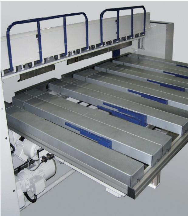
Motorized back gauge, converter-controlled
