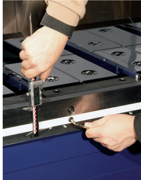
For the fine tuning: crowning system
