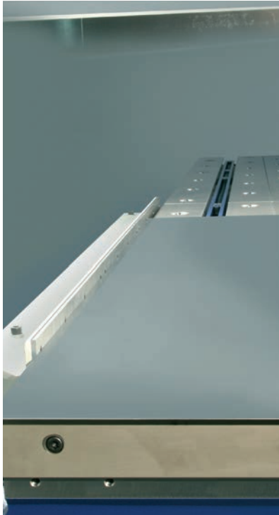
Side gauge: The precision of forming starts with an exact positioning of the workpiece. Standard with U- and J-gauge.
