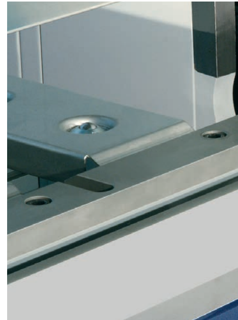
The lowerable folding beam is necessary to bend bigger radii with high precision. As an option, a motorized folding beam adjustment is available, controlled by the graphic control POS 2000 Professional.
