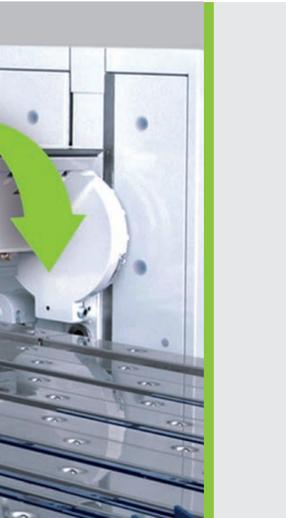
With a rotating clamping beam the MPB keeps a second set of tools in readiness.
