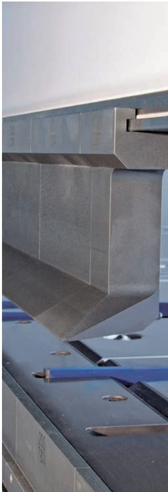
Segmented goat's foot blade, hydraulic tool clamping
