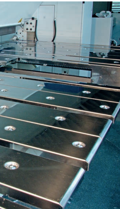
U-gauge with balls in the table for better sheet handling
