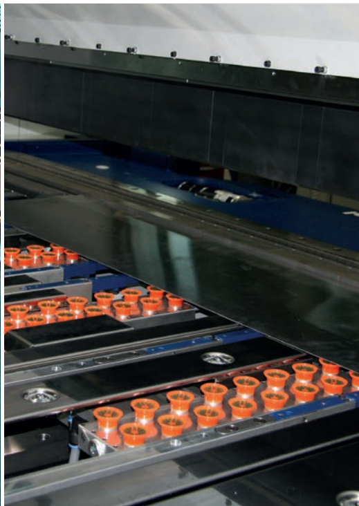
With the optional suction gauge all bends on one side can be done with one simple move by the operator
