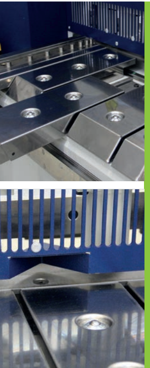
Finger guard with recessed grips
