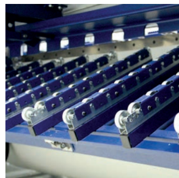
Sheet support, pneumatically controlled
