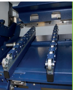
Sheet support, pneumatically controlled
