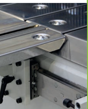
Moveable table extension on guide rail
