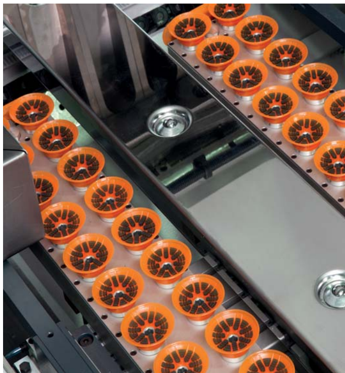
Suction plates in gauge table with 4 suction units (from 3200 mm with 6 suction units), controlled via the software POS 3000.
