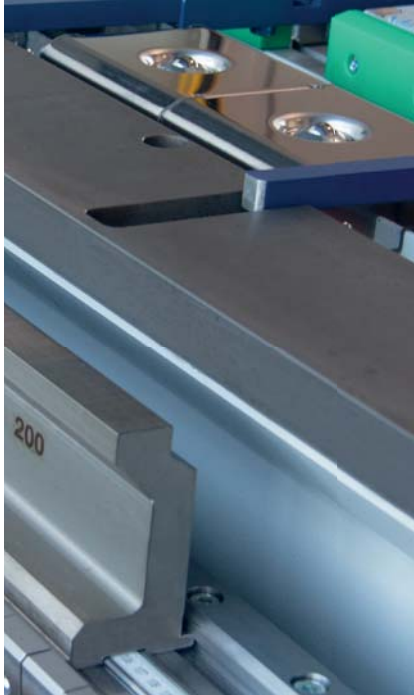
Bottom beam blade with finger grooves
