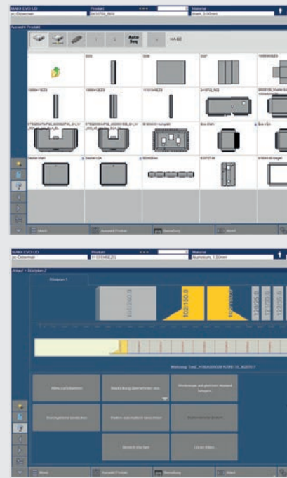
Above: The control software becomes a convenient product catalog. Below: Not only the work piece is displayed, the tools are also shown – in this case, in the mounting plan.
